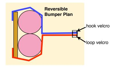
Step 7: Assembling the bumpers. Cut the pool noodles to the right length. Pool noodles cannot be hot glued together, but they can be taped or superglued.
