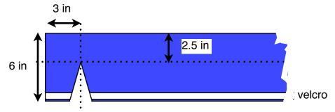
Step 9: *Finishing*. Attach the aluminum angle to the top and bottom of each bumper. Attach the adhesive velcro to the aluminum angle. Attach the hook velcro (hard) to the aluminum angle on the red side. Attach the loop velcro (soft) to the aluminum angle on the blue side. The bumpers are now reversible!
